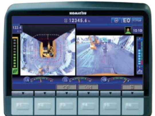
Improved monitoring system with KomVision surround view system as standard. Eco gauge, eco guidance and fuel consumption gauge help to further reduce consumption.
