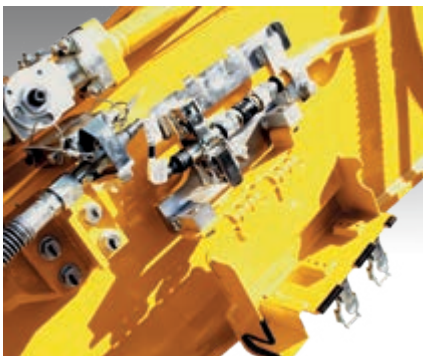
Quick release waterproof electrical connections are protected by strong flip down cover
