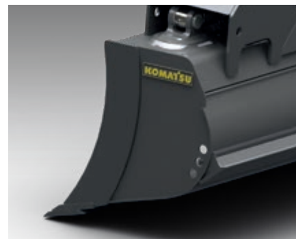
Compact S shape Round, compact shape for excellent fill values and easy discharge of material. Optional rear blade available. Reversible bolt on front cutting edge is standard on all ATB.
