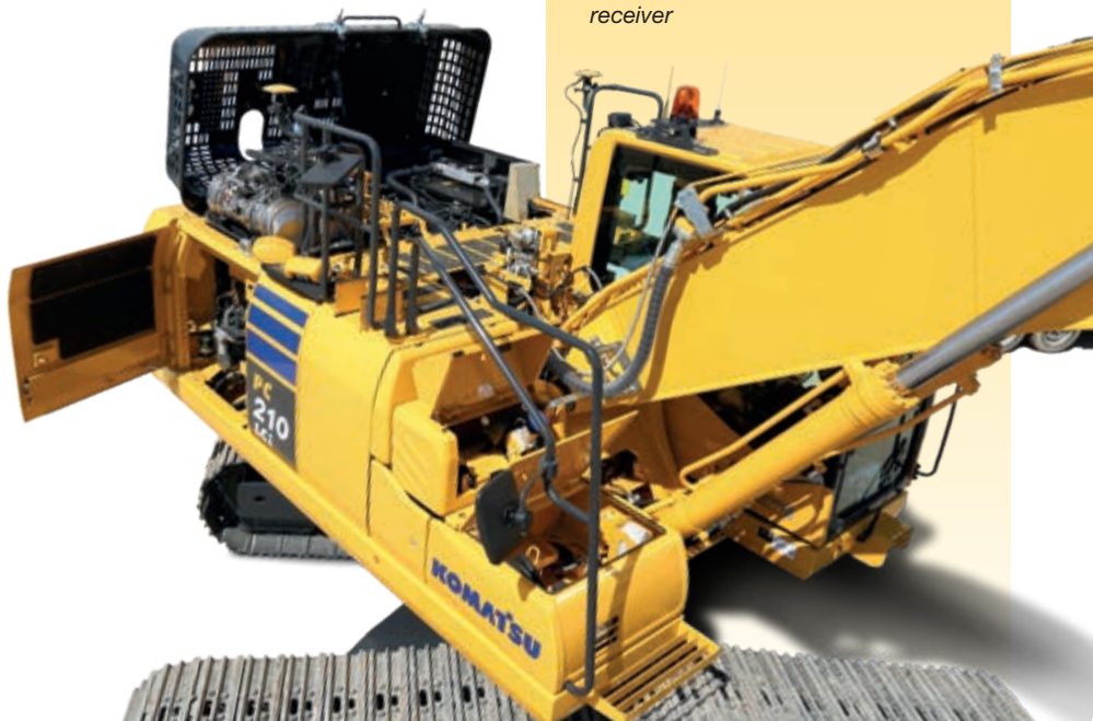
Easy access to reset MC-R3 receiver
