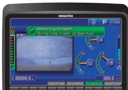
Eco-gauge, Eco guidance and fuel consumption gauge
