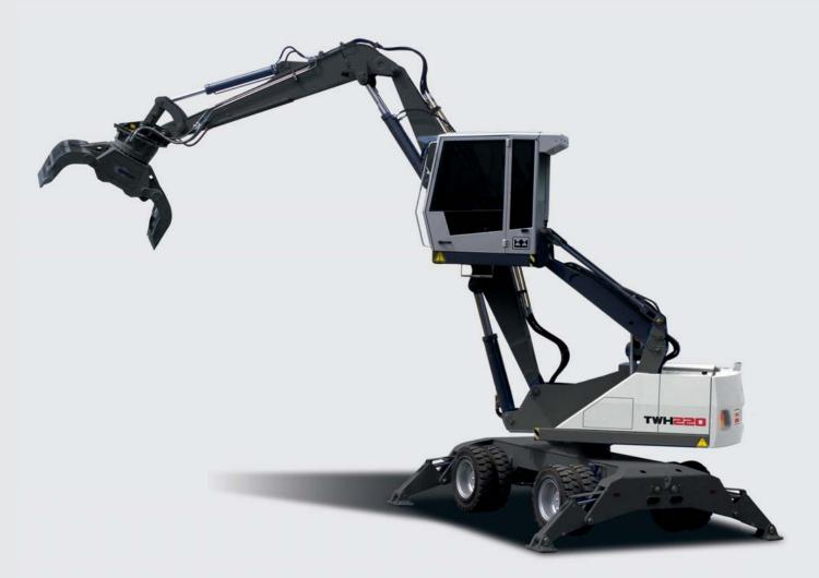
Compact, maneuverable, powerful: a snapshot of the mobile material handler TWH220. With a reach of 9.2 meters and an operating weight of 19 tonnes, this machine is the ideal solution for those who refuse to compromise on performance, efficiency and reliability – even in an entry-level model.
