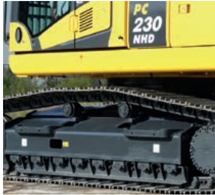
Narrow heavy duty undercarriage and narrow upper structure
