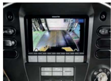
Fully integrated rear-view camera system
